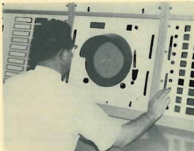
An EROS ground station operator locates an aircraft by pressing button and watching radar blip "bloom" on screen.
