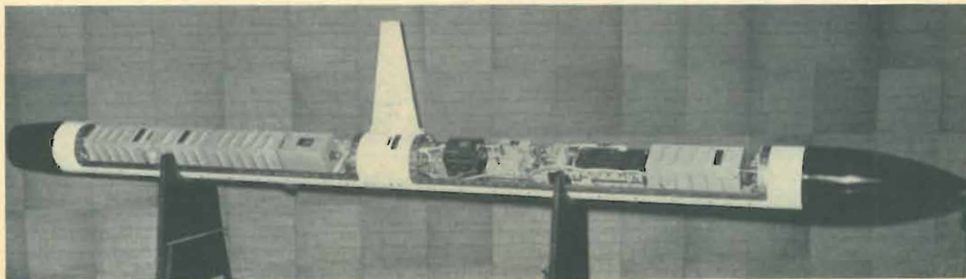
Collision avoidance pod with access doors removed to show packaging of electronic components in Sparrow III guided-missile shape.
